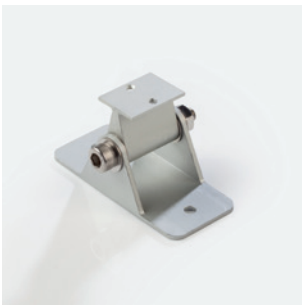
KKBK-16 Small adjustable bracket (allow 2 per metre/40in) Silver anodised aluminium finish Pre-assembled for double tail
